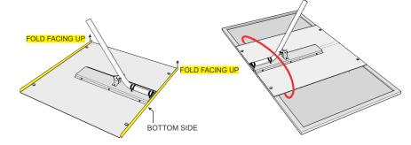
3. Install the larger plate to the narrow plate. The Fold of the plate should be facing upwards.
