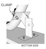
2. Install one T Section to the narrow plate, The bolt head should be on the bottom side with the threads facing upwards.
